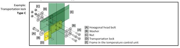
Remove the side panel on the temperature control unit to loosen and tighten the transportation locks.
