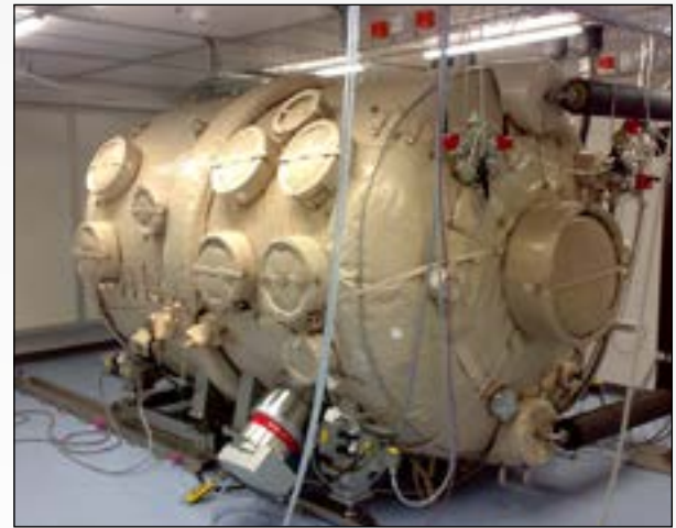
The chamber is insulated suitably for a clean room
